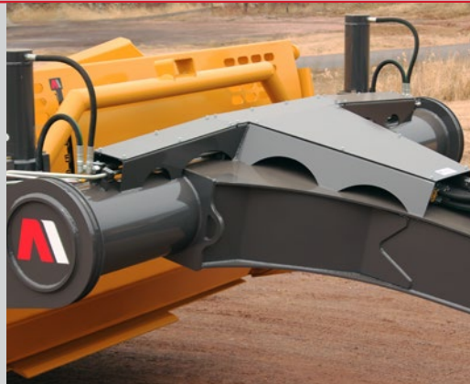
Torsion Box Style Reinforced Hitch Pole
