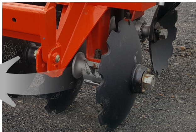
Rod stops to adjust the gang angle
