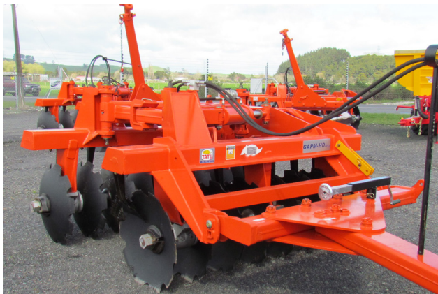
Articulated drawbar for easier transportation
