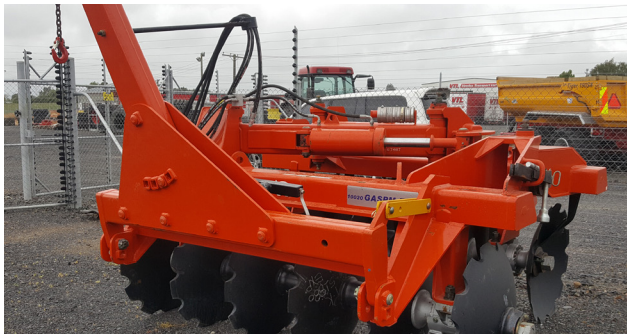
Articulated drawbar for easier transportation
