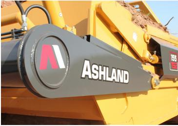
The Pole is comprised of two formed high grade steel plate halves. Add our thick wall front pipe and it's the strongest unit out there.
