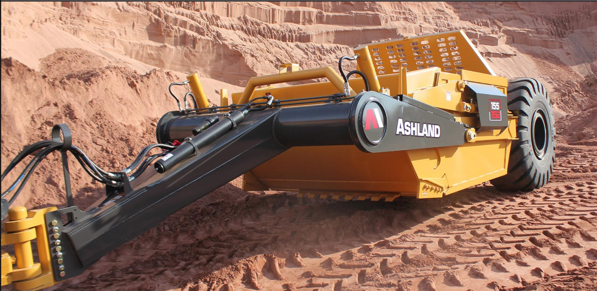
The 155TS2 sets the standard for this class of machine. Most notable are the standard features: an ejector cylinder with a thicker rod and barrel, large tires to run through anything, and beefed up trailing arms that will take the abuse.
